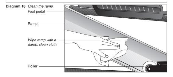
22. **Clean the ramp.** Diagram 18. Wipe down the ramp and foot pedals with a soft cloth dampened in a diluted solution of mild soap and water.
